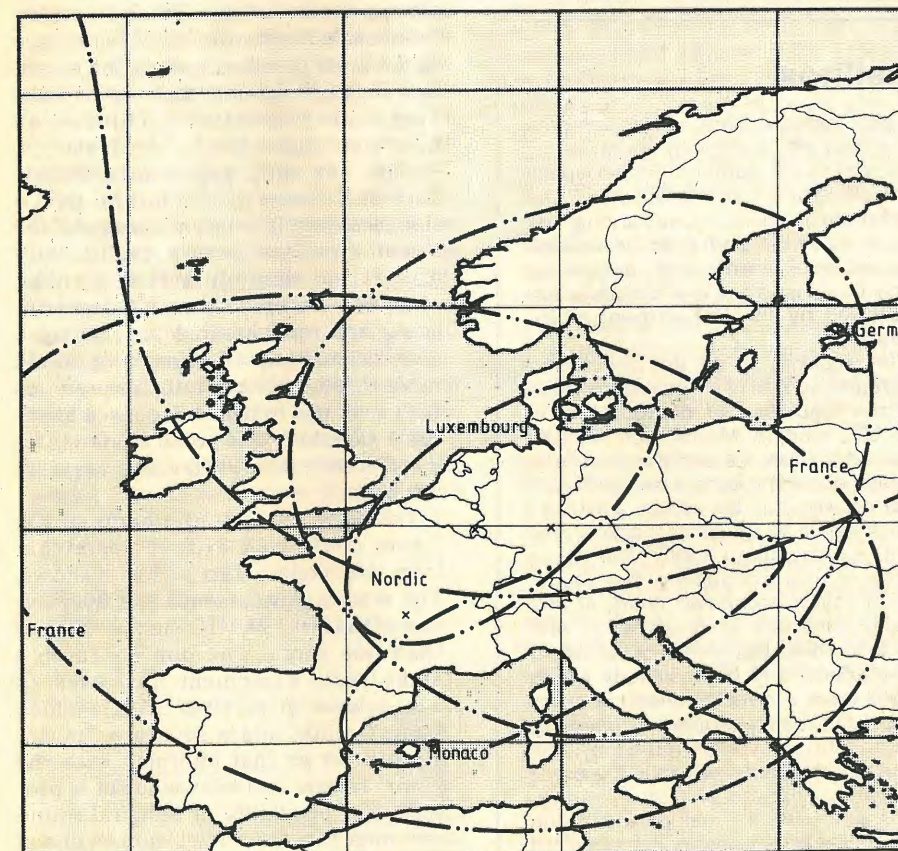
Fig. 3. Coverage area for reception on a larger antenna (1.8 to 2.0m diameter), for countries given in Figs. 1 and 2. Flux density is -111\text{dB(W/m}^2\text{)} .
